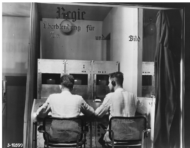
FIGURE 5 The Telefunken television studio at the Fair with the mixer for the cross-fading between film and live-pictures. Source: AEG-Telefunken Archiv, Deutsches Technikmuseum Berlin, signature AEG HA 414.
