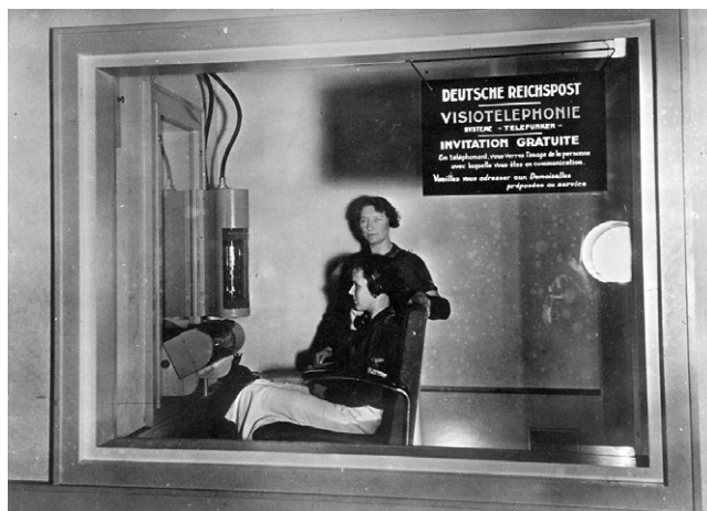
FIGURE 4 The 'Visiotelephonie'-system of the German Post Office in Paris. Source: AEG-Telefunken Archiv, Deutsches Technikmuseum Berlin, signature AEG FS 128-1-57.
